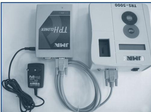
Fig.2. Example of steps 1 and 2 for connecting TPH Cloner and TRS5000.
