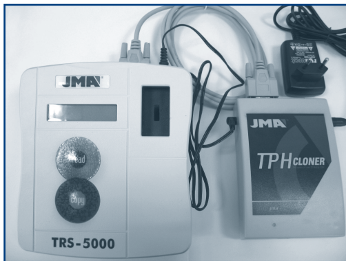
Fig.3. Example of final connection, ready for cloning.
